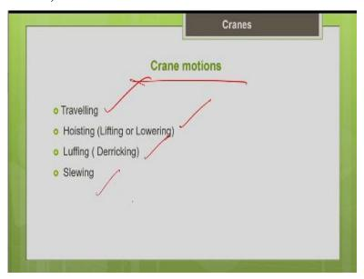
So, what are the different types of motions possible with the crane? One is your traveling, hoisting, luffing and slewing. So, basically, traveling you know for the mobile cranes, everyone knows about the mobility of the crane. Then what is this hoisting? You can either lift the load or lower the load with the pulley and drop mechanism. You can lift it or lower it that is called as hoisting. So, the other motions are luffing and slewing. We will see that.
