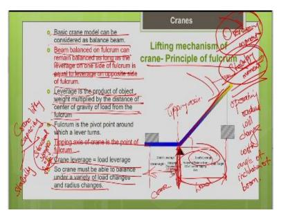
So, let us look into the lifting mechanism of the crane. What is the basic principle of lifting mechanism adopted in the crane? It is based on the principle of fulcrum. So, your basic crane model can be considered as a balanced beam. The similar to the balance beam model, you can consider your crane model also. So, I hope you remember about the balance beam and the principle of fulcrum which you might have studied during your schooling.
