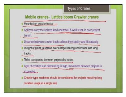
So, your lattice boom crawler crane, it is mounted on the crawler trucks as you know. So, it has the ability to carry the hoisted load, travel and work even in poor project terrain because of the track mounting. You can vary the distance between the crawler tracks which will affect the stability and the lifting capacity. So, the weight of the crane is spread over a larger bearing and the wider and longer tracks.
