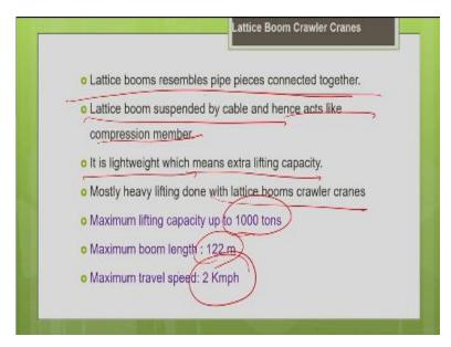
Your lattice boom basically, you know what is lattice boom, it resembles pipe pieces connected together. So, this boom is suspended by cable as you have seen in the picture and it acts like a compression member. The boom is, it is not a solid boom. It is lightweight boom. So, which means you get additional extra lifting capacity. So, whenever you want heavy lifting, we prefer lattice boom crawler cream.
