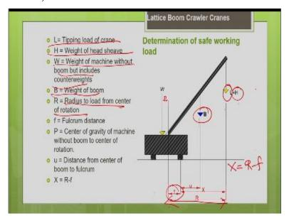
Now, let us see how to determine this safe working load for this mobile crane. So, basically as I told you, there are 2 moments acting on a crane. One is the overturning moment. Other one is your stabilizing moment or the resisting moment. So, we need to balance these 2 moments for the stability of a crane. So, accordingly, only we will choose the counter weights, everything the needle for a particular crane.
