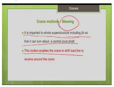
Then about the slewing motion of the crane. So, as you know, you have the slewing ring or the turntable which will give you 360-degree rotation. So, with that I can revolve my load length around the crane. It is imparted to the whole superstructure including the jib. So, that it can turn about a central pivot shaft. So, this slowing motion enables the crane to shift the load line to revolve around the crane.
