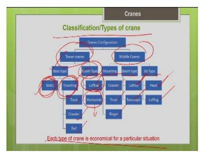
Now, let us look into what are all the different crane configurations possible. Different types of cranes are available. You can classify it from different perspective. So, basically, the crane is classified into 2 important categories based on mobility. One is mobile crane; other one is tower crane. So, when compared to mobile crane, your tower crane has relatively lesser mobility.
